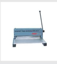
Table top guillotine intended for use with both foil and metal based photopolymer printing plates. Designed for optimum burr free cutting. Max. cutting width: 650 mm (25.6") Max. plate thickness: 0.5 mm (0.02") Max. carrier thickness: 0.3 mm (0.012") Dimension (WxDxH): 848 x 454 x 295 mm (33.4 x 17.9 x 11.6") Weight (approx. net): 72 kg (159 lbs) (ca. brutto): 100 kg (220 lbs)
