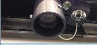
HD Ethernet Cameras to enable the highest quality register mark image
